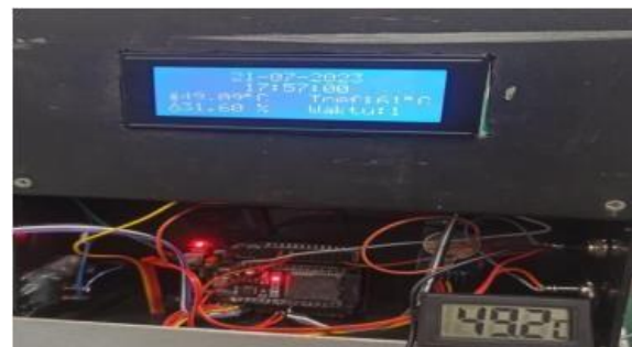
Figure 3. Comparative testing of DHT22 and digital temperature.
