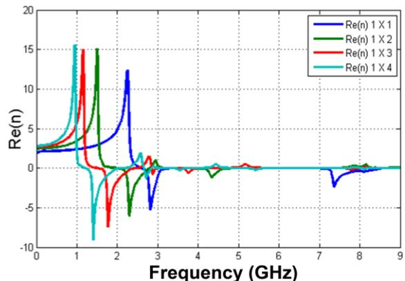
**Figure 7.** Refractive index graph metamaterial 1 – 4 SRR-Circle.
