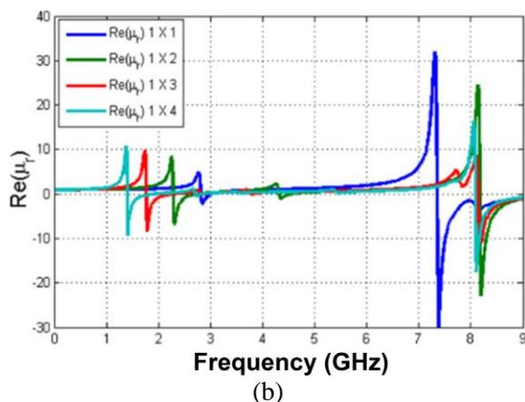
**Figure 6.** Graphs (a)  $\epsilon_r$ , and (b)  $\mu_r$  of metamaterial combination 1 – 4 SRR-Circle.
