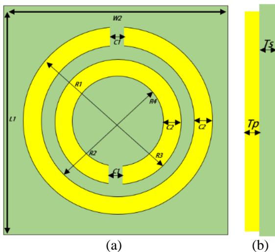
**Figure 3.** SRR structure: (a) front and (b) side.
