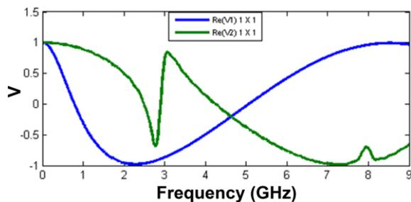
**Figure 5.** Graph of the real part V1 and V2 of the FR4 substrate ( $\epsilon = 4.3$ ).
