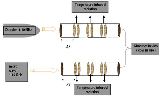
Figure 3.1. A schematic diagram of the process in a photo acoustic cell for cow cancer cell tissue in experiment using range of frequencies in MHz and GHz
