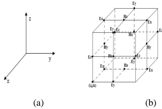
Figure 3.2. Yee cell shows the spatial and radial (a) relationship of  $E$  and  $H$ . (b)
